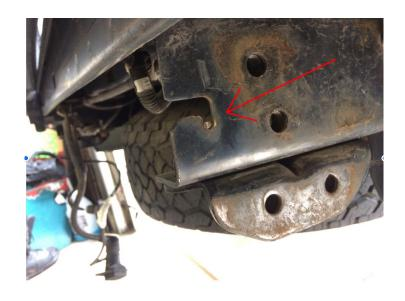
Install factory license plate light housings into new bumper using the supplied #8 machine screws, washers, and nuts.
