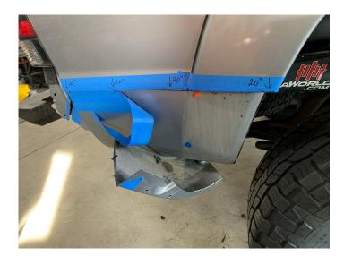
Remove any burrs from your cut edge with a file and paint the edge to protect from corrosion.
