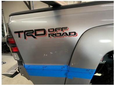
the bed yet, it will help to leave this installed to stabilize the bed while cutting. Always wear proper protective equipment such as safety glasses, face
