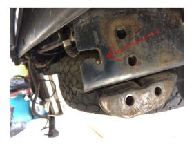
If you are installing backup lights, it is easier to bolt them on with the bumper off the truck but can can be done after the bumper is installed as well. The holes are cut for any brand flush mount LED pods. Wiring is up to you, but it is best to use a relay switch powered directly from the battery and use the reverse light circuit as it's trigger. Using the
