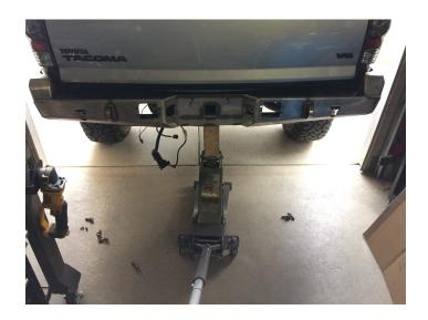
\*Note\* Tacoma beds are all set slightly different from the factory. You can slightly adjust the bed left/right by loosening the six T55 torx bed bolts and sliding it either way.
