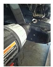
Using a 1/4" bit, drill out the aluminum rivets holding the factory turn signal brackets and remove them.
