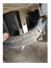
Carefully remove the plastic connector holding the power steering cooler line into the radiator support
