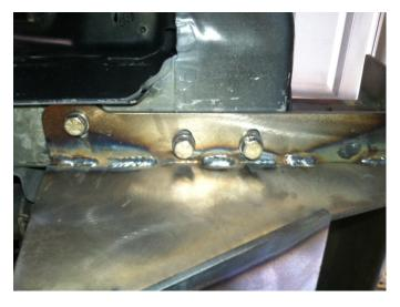
Insert provided bolts into the existing factory holes and thread in all six bolts about half way. After all six are in, check side to side alignment as the mounting holes are slotted for adjustment. The bumper can also move front to back slightly. Now tighten all six bolts.
