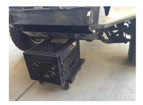
Now carefully slide the bumper into position. Using a floor jack or moving dolly with crate/ lumber will make positioning the bumper a lot easier. The power steering cooler lines slide into the slot cut for them on the radiator skid.
