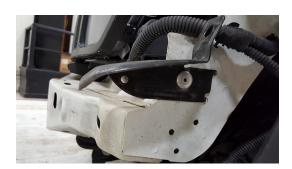
If your KK was equipped with a factory radiator skid, it must be removed. Your new ATH bumper includes a much better radiator skid. Also remove tow hooks if they are present.
