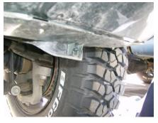
Once those are gone cut the pom rivets that secure the splash guard to the bumper
