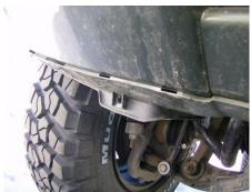
Now comes the hard part. There are 3 butterfly plastic spring clips that hold the front of the flare to the bumper. If you snake your hand behind the bumper from the bottom, you can release the bottom one. Once you get that one, either use a small pick and try to release each finger on the other two, or use a small pich and try to release the clip from the flare. If you do the latter of the two, depress the little nubs and push the clip towards the rear of the KK.
