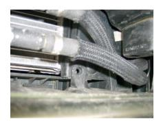
Move to the front of the KK and remove the 2 push pin style fasteners that are located by the P/S cooler
