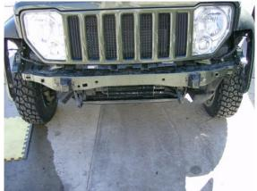
Upon reinstallation, the permanent plastic rivets that were drilled out can be replaced with reusable plastic push pin rivets (the same style used on the splash guard).
