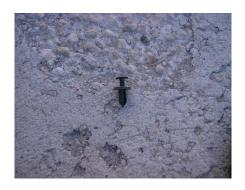
Next remove the 3 fasteners that hold the splash guard to the bumper. They pop open like this.
