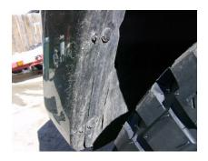
First using the pick tool, push out the center of the 2 pom rivets that secure the rear of the fender flare to the bumper. These can also be drilled out and replaced with push pin rivets.
