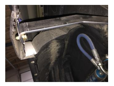
4. Now install new bumper. It may help to have a buddy's assistance in lifting. Lift bumper in place and slide into the two rearmost bolts you left halfway threaded in. It is helpful to place a floor jack with wood blocking under the receiver to lift and hold it in place. Thread in the other 8 bolts you removed earlier but leave loose.
