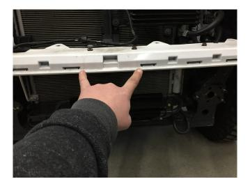
2. Disconnect the fasteners holding the thin plastic wheel well liners/splash guards up to the point the bumper meets the fender and fold the liner back out of the way for now. Disconnect the fog light wiring harnesses from the back of the fog lights. Remove plastic fog light trim bezels by pulling forward firmly and prying with plastic trim tool. Do not remove plastic bumper cover just yet.
