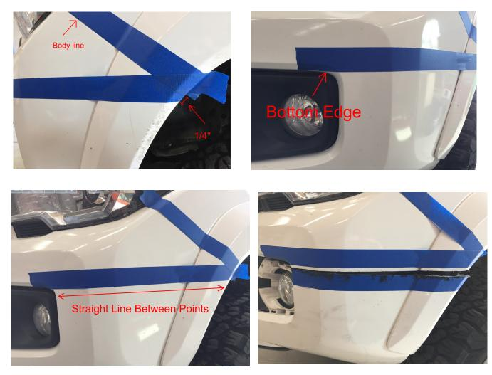
Double check your tape lines and make your cuts a 1/4" <u>below</u> the bottom edge of the horizontal tape line. This will give you room for error, and you will be mounting the bumper up tight against this cut line later to check your final cut line. Also cut along the top of the plastic fog light pockets where they connect to the bumper cover.
