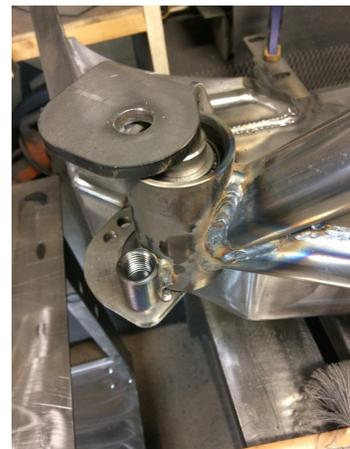
Install spring loaded pop pin into the threaded barrel on the bearing housing.
